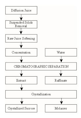
Raw juice is obtained in the usual manner via diffusion. Suspended solids must be removed from the raw juice in order to prevent plugging and pressure drop in the softener and the chromatographic separator.
