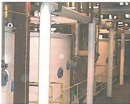
Figure 2. A simulated moving bed system for chromatography of beet molasses
